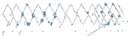
Fig#17 Combine stress Loadcase DL+Wind+Lateral OP + Lift cable failure
