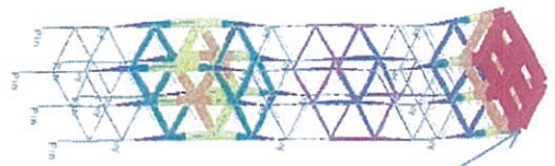
Fig#8 Deformation Uy Loadcase DL+Wind+Lateral OP
