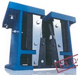
VI Safety Gear E3 policy complied safety components --- Passed 25 times freefall and runaway test without component replacement.
